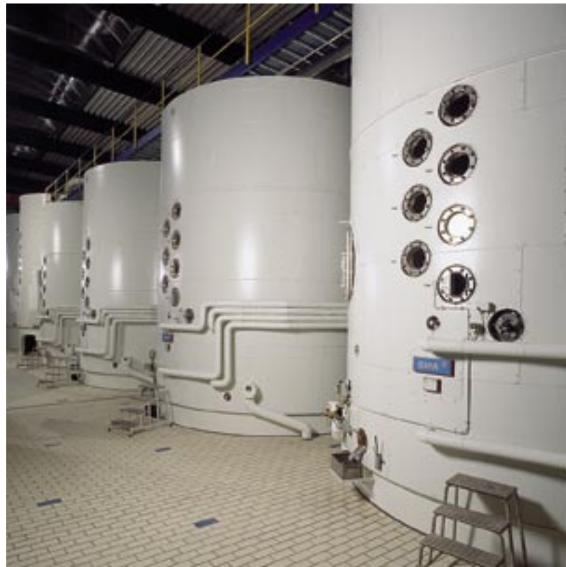
Batch pans for 1st and 2nd white massecuite
